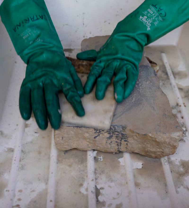
Limestone from Cantanhede cutted and leveled by Antonio Régis da Silva and grinded by Catarina Marques da Cruz.
