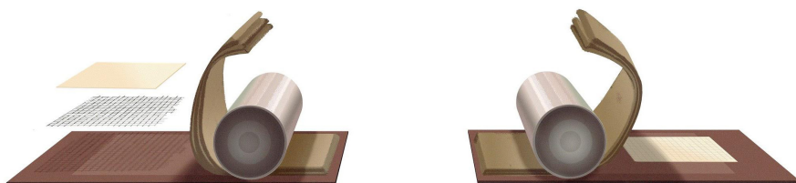
Fig. 3. Embossing process of texturing paper gaining grain, lines, nets, etc. with the usage of the printing press.
