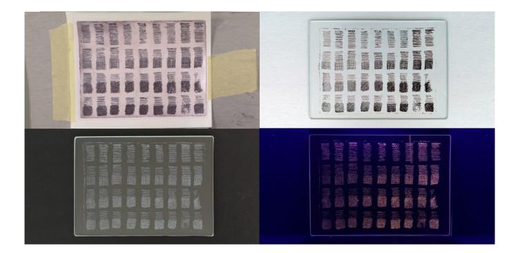
Figure 3. Intaglio samples. Views from the copper metal plates, printing on cotton paper, transfer printing on glass with black enamel and transfer print on glass with sodalite photoluminescent enamel
