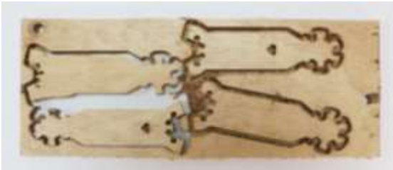
Fig. 1. CNC cut component from plywood
