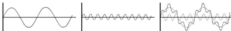
Figure 4 - Waves summation: two frequencies, two amplitudes and the resulting wave. Adapted from Waveforms: Adding waveforms and Phase (Mannell, 2008)
